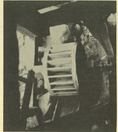
1.) Sawmill, Telemark, Norway. Looking down on the undershot wheel. The pitman arm on the right is connected to the crank of the wheel shaft and operates the saw frame.
