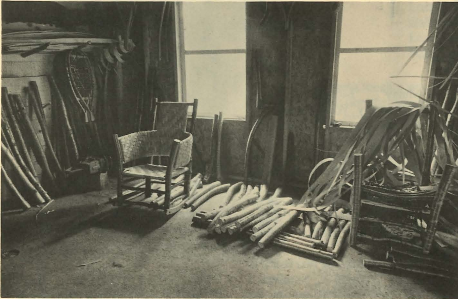
The Drying Room of Jack Leadley's Shop. On the left is a finished Fountain chair, and on the right a chair frame waiting for its black ash seat and back. The short pieces of unpeeled yellow birch on the floor and stacked against the wall must dry for a year before they are ready to make into the frames of chairs.
