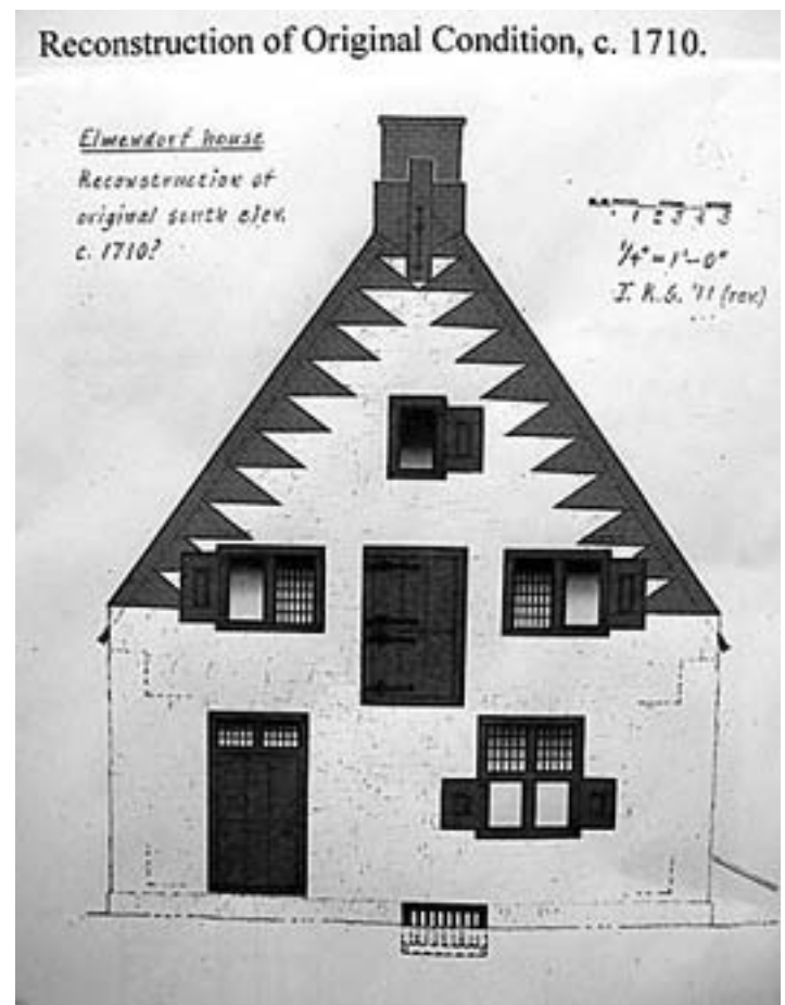
Fig. 3 (below) – Elmendorf House, Hurley, NY. Reconstruction of south elevation. Drawing by John Stevens.
